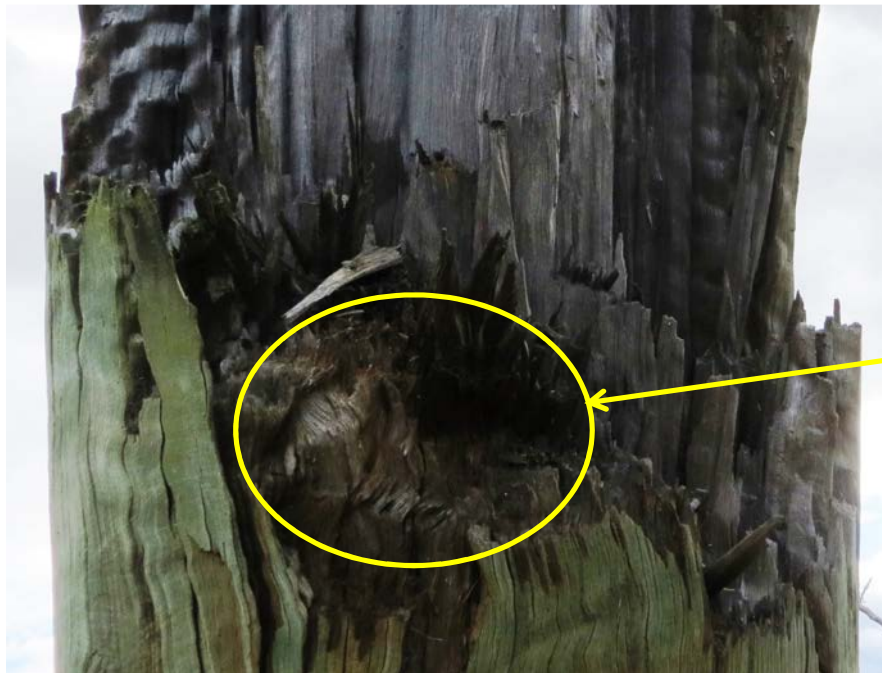
Photo 20 – Close up of pole fracture from the east showing signs of compression of fibres.
